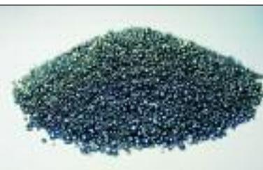
**Silicon granulate from a fluidised bed reactor**
