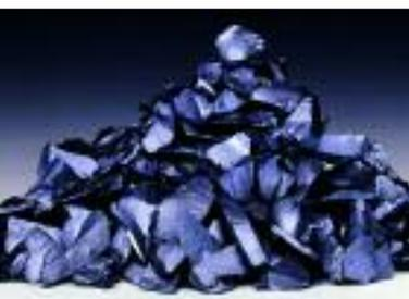
**Broken silicon rods: The feed material is melted down again and then, with the help of a seed crystal, extracted from the melt as a cylindrical single crystal.**
